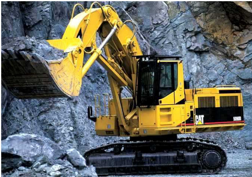
Front shovel, track-mounted Hegybontó, lánctalpas
