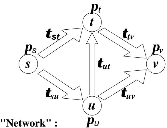
Connected weighted directed graph with a single source and a single sink but with no loops and no negative weights.
