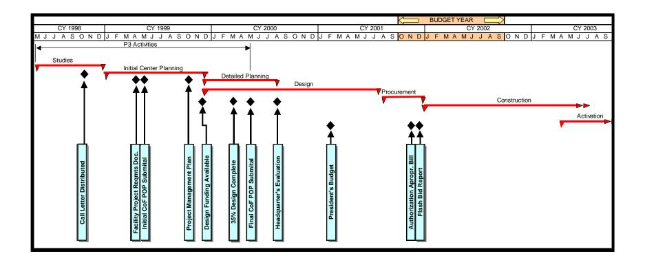
Figure 3.1 Typical NASA Construction of Facilities (CoF) Project Cycle
