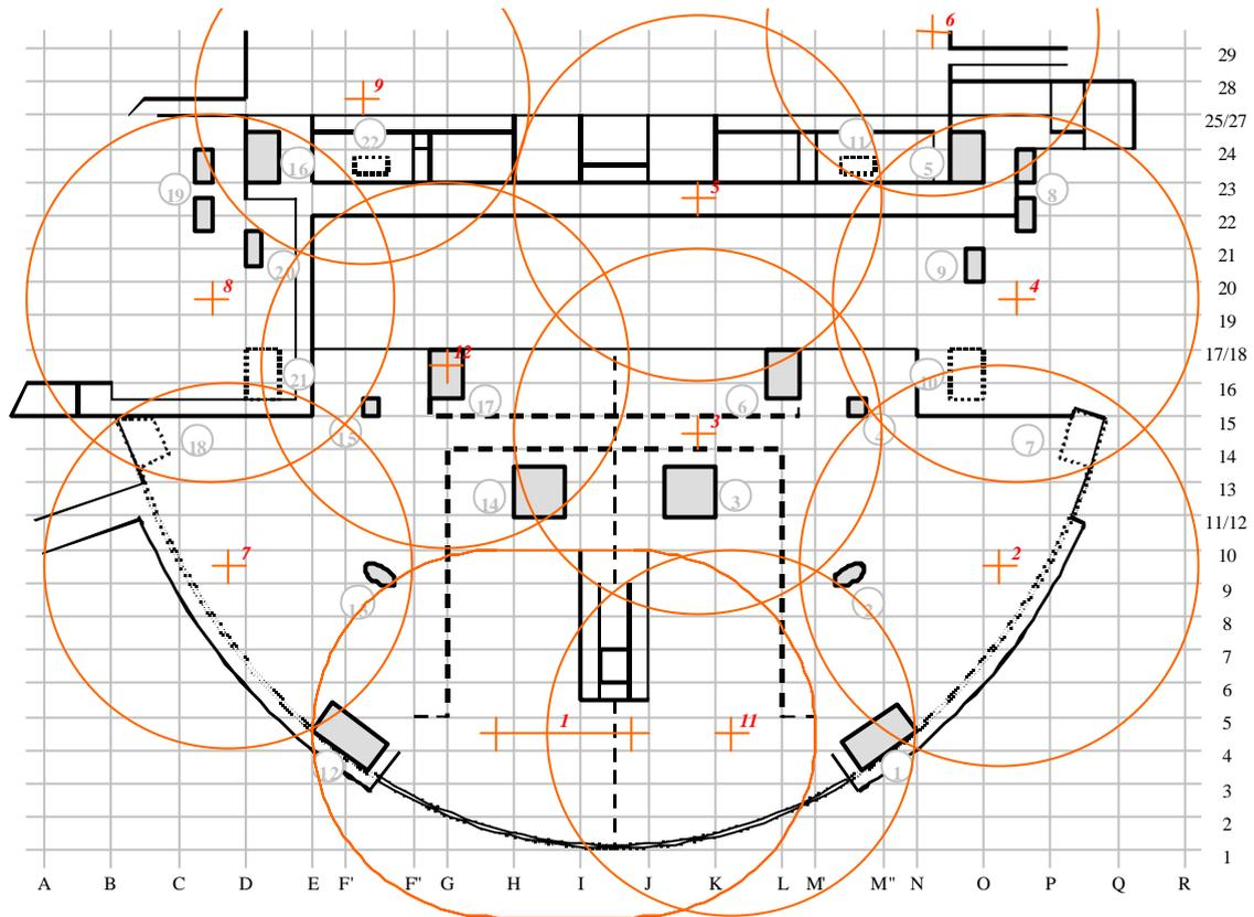
**Picture 1.;** Asia Center, Construction Phase I. ( „Son” and „Daughter” Buildings ) structural works, Crane layout plan ( STRABAG Building Ltd. 48. Dir. )
