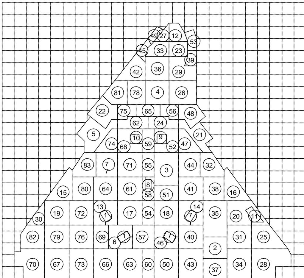
**Picture 2** Asia Center, Phase II. („Father” Building ) water proof R.C. foundation slab, block design and schedule proposal ( to be approved ). Background grid reflects 8 x 8 m raster of piers.
