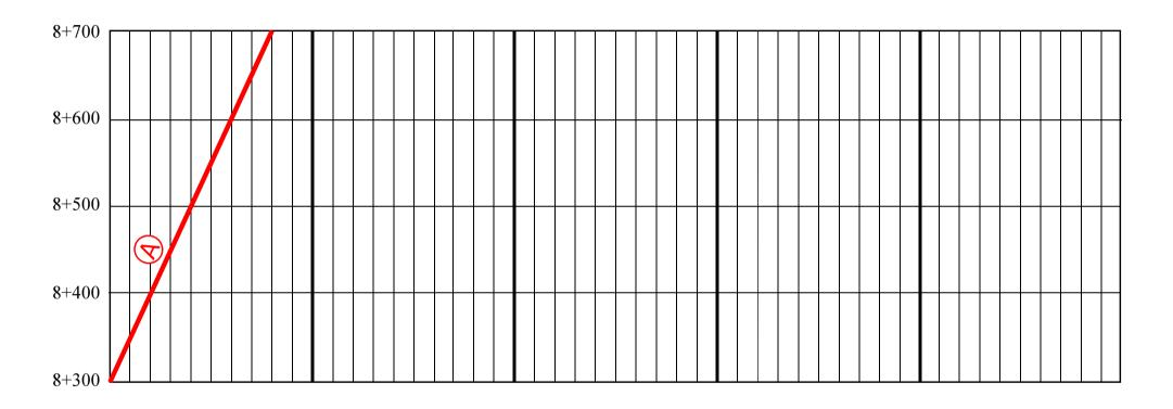
Activity "A" is to be performed all along the whole 400 m long section. The job is performed by one team, with constant, 50 m/day intensity, advancing from section 8+300 to direction of section 8+700. Performance starts on day 1 and finishes on day 8. Scheduled duration is 8 days.
