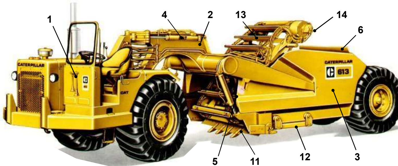
All-Wheel-Drive Scraper (Charging and penetration provided by towing power of tractor)
