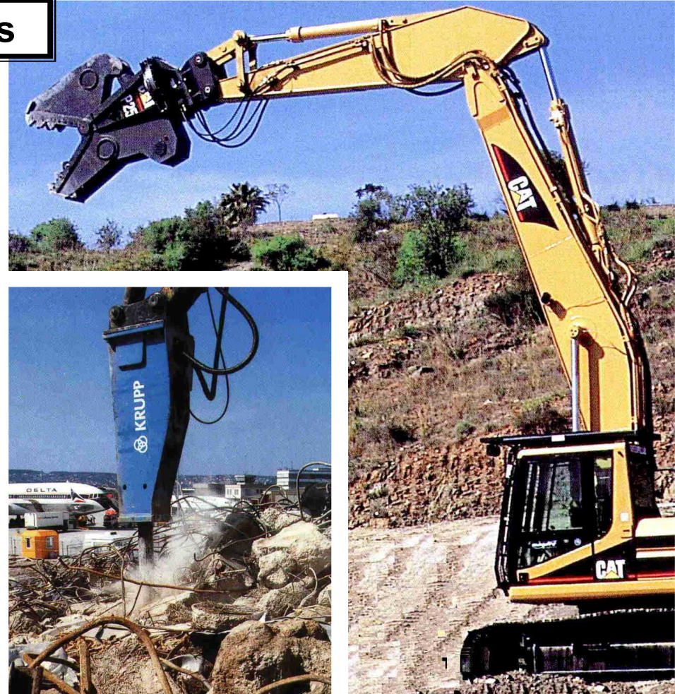
Breakers, Jaws (for concrete, reinforced concrete and steel)
