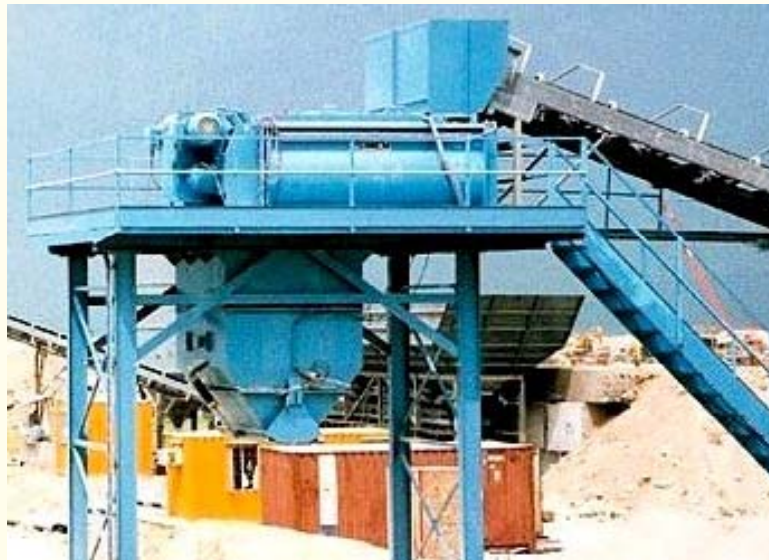
Concrete delivery (through collector basin)
