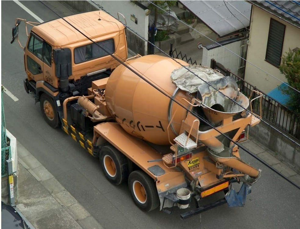
Mixer truck (charger chute open)
