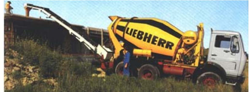
Mixer truck with delivery conveyor (in action)
