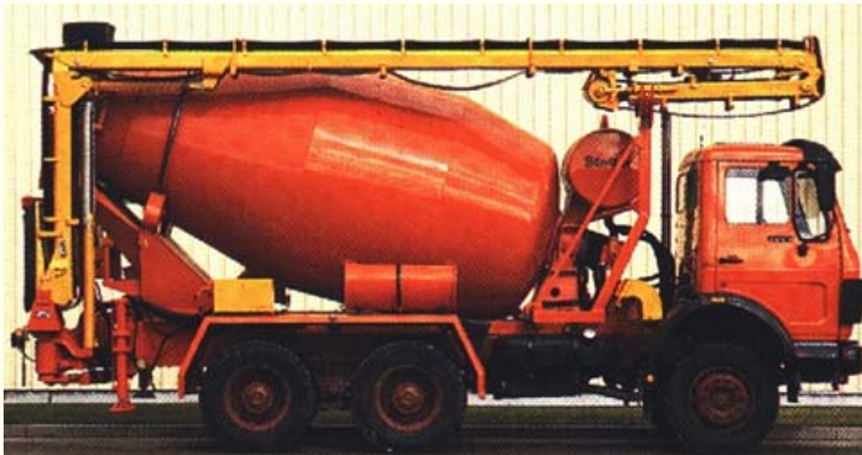
Mixer truck with delivery conveyor (riding position)
