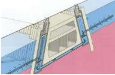
Cut-and-cover methods for metro stations
